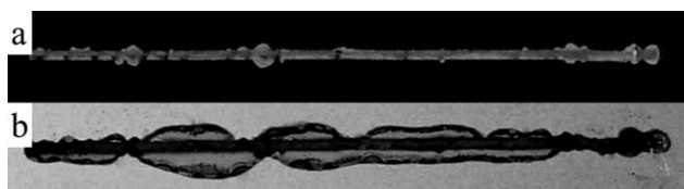
Fig. 5. Photographs of scratches on the cured 1 wt% EB/DGEBA/TMDA samples made using Route A . (a) Before the immersion test. The coating is dark. (b) After immersing 17 days in 3.5% NaCl the coating has been removed and the average width of the scratch is wider than in the beginning.
